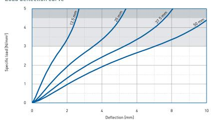
Recording of the 3rd loading; testing between steel plates with emery cloth of granulation K 120 at room temperature measured at  $v = 0.2 \text{ N/mm}^2 / \text{sec}$
