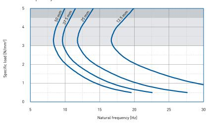
Natural frequency of a single-degree-offreedom system consisting of a fixed mass and an elastic bearing consisting of PURASYS vibradyn HL 3000 on a stiff subgrade.
