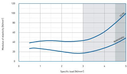
Dynamic test: sinusoidal excitation with an oscillating range of  $\pm$  0.11 mm at 10 Hz
