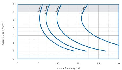
Natural frequency of a single-degree-offreedom system consisting of a fixed mass and an elastic bearing consisting of PURASYS **vibra**dyn HL 6000 on a stiff subgrade.
