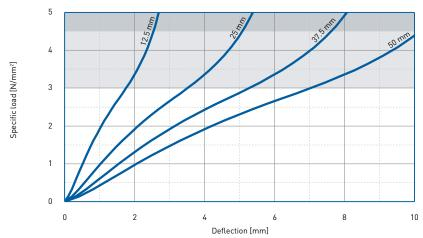
Recording of the 3rd loading; testing between steel plates with emery cloth of granulation K 120 at room temperature measured at  $v = 0.2 \text{ N/mm}^2$  / sec
