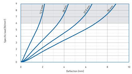
Recording of the 3rd loading; testing between steel plates with emery cloth of granulation K 120 at room temperature measured at v = 0.4 N/mm<sup>2</sup> / sec
