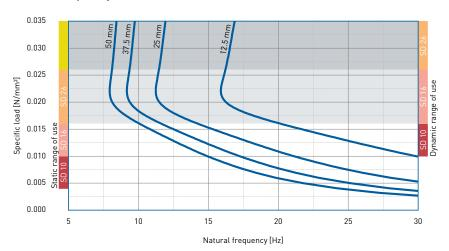
Natural frequency of a single-degree-offreedom system consisting of a fixed mass and an elastic bearing consisting of PURASYS **vibra**foam SD 16 on a stiff subgrade.
